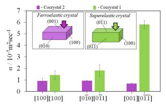
**Fig. 5** The obtained thermal diffusivity values of cocrystals **1** (light green colored) and **2** (purple colored) with respect to the longer, wider, and thinner axes, respectively. Arrows indicate the direction of shear stress deformations.
