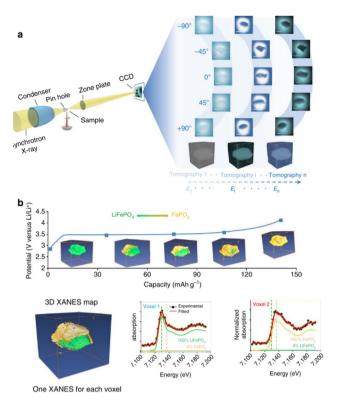
Fig. 11 Illustration of a 5D Fe K-edge XANES tomography. (a) Schematic of the experimental setup. A tomography data set is collected at different energies across the near Fe K-edge absorption to access chemical information for each voxel. By fitting the resulting spectra as a linear combination of spectra of end-phases, phase composition can be assigned to each voxel (right side). (b) Chemical phase distribution as a function of capacity (proportional to time). Reproduced from ref. 154
