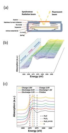
Fig. 6 (a) Scheme of coin cells allowing measuring S K-edge *operando* in fluorescence mode. (b) Sulfur K-edge XANES evolution as a function of the state of charge followed *operando* in Na/S batteries and (c) selected spectra at various states during the first cycle with positions for reference compounds highlighted by vertical dotted lines. Reproduced from ref. 19, © John Wiley&Sons.
