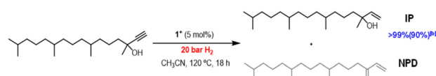
Fig. 6 Semihydrogenation of DIP. Reaction conditions: 0.1 mmol alkyne, 5 mol% catalyst, 20 bar H 2 , 120 °C, CH 3 CN (2 mL), 18 h. Conversions and yields determined by GC analysis using n -hexadecane as an internal standard.
