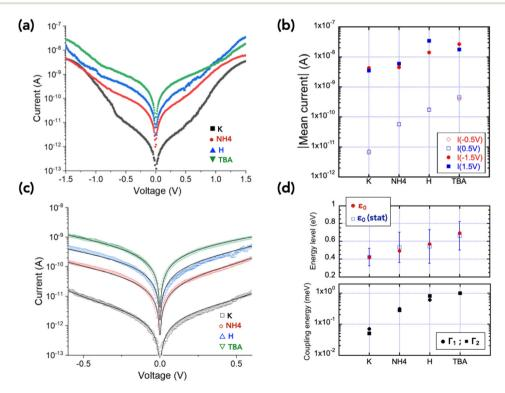
Fig. 3 (a) Mean  $\bar{I}-V$  curves for the four samples (from the datasets shown in Fig. 2), (b) counterion dependence of the mean current  $\bar{I}$  at  $\pm 1.5$  V and +0.5 V, (c) fits (solid lines) of the SEL model in the voltage window [-0.6 V; 0.6 V] (fit  $R^2 = 0.995$  for  $K^+$ , 0.998 for  $NH_4^+$ , 0.995 for  $H^+$ , 0.999 for TBA<sup>+</sup>), (d) evolution of the SEL model parameters  $\varepsilon_0$ ,  $\Gamma_1$  and  $\Gamma_2$  with the counterions.
