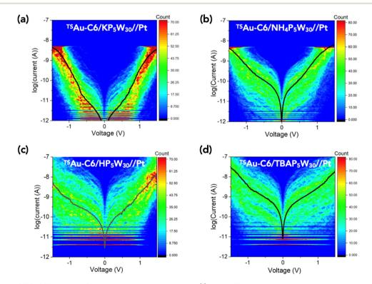
Fig. 2 2D histograms ( $400-500\ I-V$  traces) of the four samples in a semi-log|I|-V plot. The solid black lines are the calculated mean  $\bar{I}-V$  curves. (a) KP<sub>5</sub>W<sub>30</sub> MJs, (b) NH<sub>4</sub>P<sub>5</sub>W<sub>30</sub> MJs, (c) HP<sub>5</sub>W<sub>30</sub> MJs and (d) TBAP<sub>5</sub>W<sub>30</sub> MJs.
