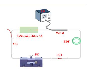
Fig. 7 The setup of a mode-locked EDF laser.
