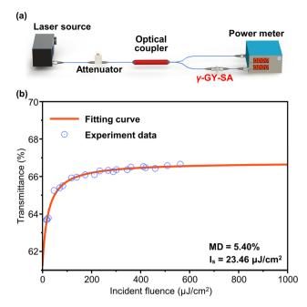
Fig. 4 (a) Schematic of the balanced twin-detector measurement. (b) Relationship between transmittance of the γ-GY-SA and incident fluence.
