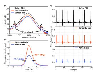
Fig. 10 (a) Spectra, (b) oscilloscope traces and (c) the autocorrelation traces of vector solitons.
