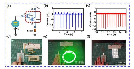
Fig. 8 (a) Schematic diagram of the MCH-TENG and a Darlington transistor connected circuit. (b and c)  $I_{\rm sc}$  of the 2# MCH-TENG without (b) and with (c) the Darlington transistor under hand tapping. (d and e) The circuit connected to different loads: (d) electronic counter ( $V_{\rm cc}$  = 5 V); (e) LED light strip ( $V_{\rm cc}$  = 12 V); (f) LED light board ( $V_{\rm cc}$  = 18 V).
