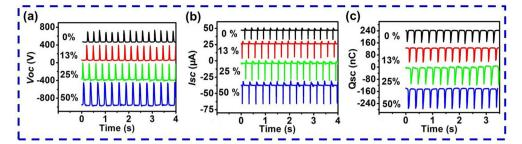
Fig. 4 (a)  $V_{\rm oc}$ , (b)  $I_{\rm sc}$  and (c)  $Q_{\rm sc}$  of the 2# MCH-TENG under stretching strain from 0% to 50%.
