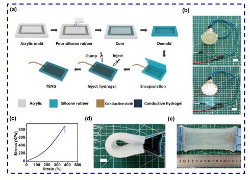
Fig. 1 (a) Schematic diagram of the detailed fabrication process of the MCH-TENG. (b) Photographs of the circuit comprising of the MCH and LED light (V = 8 V; top: open circuit; bottom: closed circuit). (c) The stress-strain curve of the silicone rubber cube ( $59 \times 10 \times 2 \text{ mm}^3$ ). (d and e) Photographs of the MCH-TENG at bending (d) and stretching states (50%). (All scale bar = 1.0 cm.)
