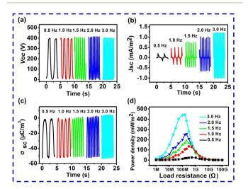
Fig. 3 Electrical output performance of the 2# MCH-TENG at different contact frequencies. (a-c) Electrical output ( $V_{oc}$ ,  $J_{sc}$  and  $\sigma_{sc}$ ). (d) Power densities under different external loads.
