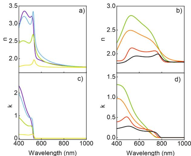
**Fig. 4** The refractive index (a and b) and extinction coefficient (c and d) calculated for the ligand-free quantum dots of different composition and size. (a and c) MAPbBr<sub>3</sub> QDs (green line, QD size: 2.4 nm; blue line, 2.3 nm; violet line, 2.2 nm) and a polycrystalline film (yellow line). (b and d) MAPbI<sub>3</sub> QDs (red line, 9 nm; orange line, 7 nm; green line, 6 nm) and a polycrystalline film (black line).
