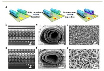
Fig. 2 Manufacture of mesostructured Swiss-roll microelectrodes. (a) Schematic of the Zn-MnO<sub>2</sub> Swiss-roll microbattery fabrication process. Top (b) and side view (c) SEM images of mesostructured Swiss-roll microcathode. (d) Magnified SEM image of the MnO<sub>2</sub> morphology. Top (e) and side (f) view of mesostructured Swiss-roll microanode. (g) Magnified SEM image of the Zn nanosheet morphology
