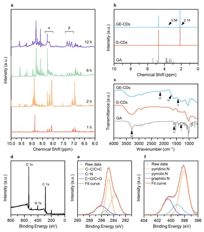
Fig. 1 (a) <sup>1</sup>H NMR spectra of GE-CDs with different reaction times. (b) <sup>1</sup>H NMR spectra of GA, G-CDs, and GE-CDs. (c) FTIR spectra of GA, G-CDs, and GE-CDs. (d) XPS spectrum of GE-CDs. High-resolution XPS spectra of (e) carbon 1s and (f) nitrogen 1s of GE-CDs.
