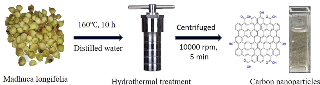
Scheme 1 Schematic representation for the one-step synthesis of the fluorescent CNPs via the hydrothermal treatment of Madhuca longifolia .
