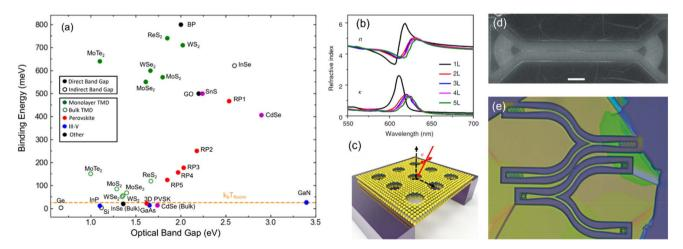
Fig. 1 Photonic waveguides. (a) Binding energy versus optical band gap of common 2D semiconductors. 5 Copyright 2022 AIP Publishing. (b) Thickness dependent refractive indices of WS<sub>2</sub>.3 (c) A schematic of the WS<sub>2</sub> photonic crystal membrane.3 Copyright 2019 Springer Nature Limited. (d) An hBN waveguide with input and output couplers.<sup>6</sup> (e) Optical image of waveguide splitter patterned on a single hBN flake.<sup>7</sup> Copyright 2021 American Chemical Society
