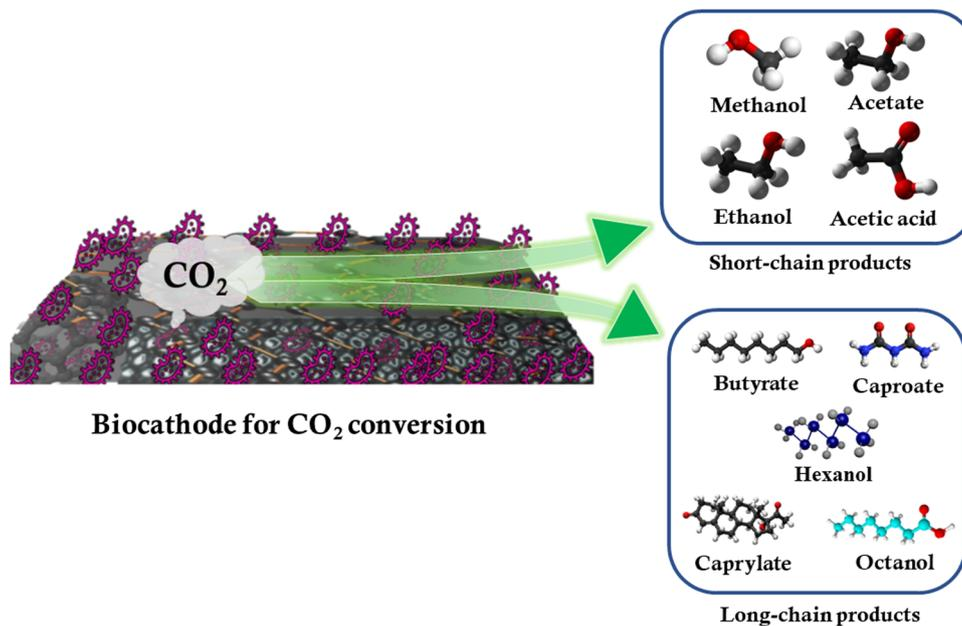
Fig. 5 Schematic of the production of various small-chain (methanol, ethanol, acetic acid, and acetate) and long-chain chemicals (butyrate, caproate, caprylate, and octanol) from CO<sub>2</sub> conversion using MES and carbon biocathodes.
