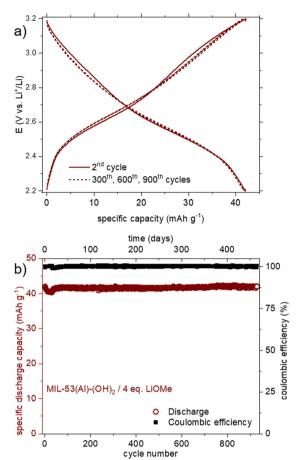
Fig. 8 a) Potential vs. specific capacity curves for the lithiation product from MIL-53(Al)-(OH)<sub>2</sub> and LiOMe-MeOH/THF. Plain lines correspond to the 2nd cycle; dashed lines to the 300th, 600th and 900th cycles; b) capacity retention and coulombic efficiency for the lithiation product from MIL-53(Al)-(OH)<sub>2</sub> and 4 eq. of LiOMe (electrolyte: 1 M LiClO<sub>4</sub> in PC; potential range: 2.2-3.2 V vs. Li<sup>+</sup>/Li).
