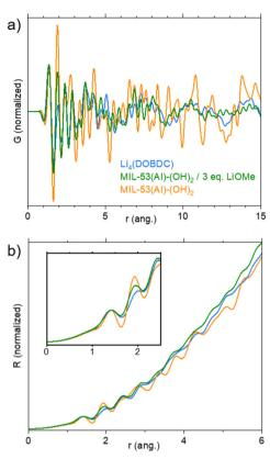
Fig. 4 Characterisation of the reaction product between MIL-53(Al)-(OH)2 and 3 eq. of LiOMe in MeOH/THF by X-ray total scattering experiments. a) Reduced pair distribution function G(r); b) radial distribution function R(r) (inset: zoom on the 0-2.5 ang. region). Data related to dry MIL-53(Al)-(OH)<sub>2</sub>, Li<sub>4</sub>(DOBDC), and the lithiation product from LiOMe-MeOH/THF, are shown in orange, blue and green, respectively.
