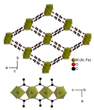
Fig. 1 Crystal structure of MIL-53(M)-(OH)<sub>2</sub> or M(OH)(H<sub>2</sub>DOBDC).<sup>20</sup> Top: View along the pore axis; bottom: view of the inorganic chain. Protons (bound to C, organic O and inorganic O) are omitted, and only one of the two disordered positions of the phenolic groups is shown.
