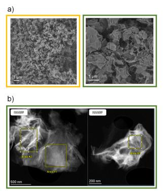
Fig. 3 Characterization of the reaction product between MIL-53(Al)-(OH)<sub>2</sub> and 3 eq. of LiOMe in MeOH/THF. a) SEM pictures of the pristine solid (left) and the lithiated solid (right); b) STEM pictures of the lithiated product. Areas used for the EDX analyses provided in Table 1 are also shown.
