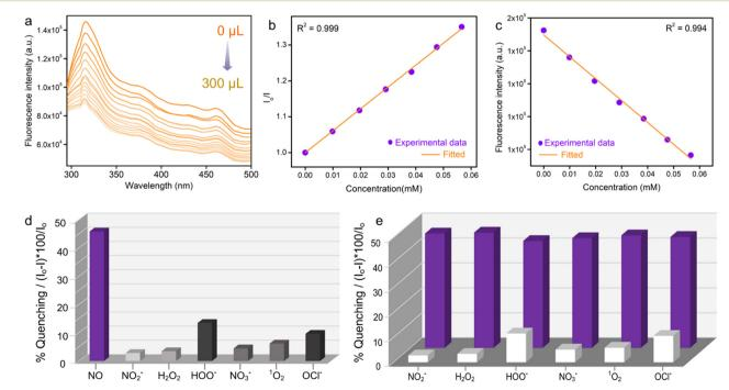
Fig. 2 (a) Photoluminescence spectra of PABA@MOF-808 in water in the presence of different concentrations of NO. (b) Stern-Volmer (SV) plots for quenching of PL intensity of PABA@MOF-808 by NO. (c) LOD calculation plot, (d) relative fluorescence quenching response towards different RNS/ROS in water, and (e) relative fluorescence quenching response towards different RNS/ROS followed by addition of NO solution.
