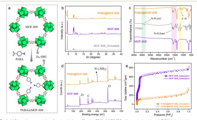
Fig. 1 (a) Schematic representation of post-synthetic modification (PSM) of MOF-808 with p-aminobenzoic acid (PABA) (colour code: grey carbon, white - hydrogen, red - oxygen, blue - nitrogen and green - zirconium). (b) PXRD patterns, (c) FT-IR spectra, (d) XPS survey spectra and (e) nitrogen gas sorption data at 77 K of pristine MOF-808 and PABA@MOF-808.
