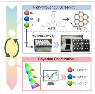
Fig. 1 Research flow process. Data were collected by changing the stoichiometric ratio of the three lanthanide metal-salts and conducting 24 or 48 variations six times using multiple reaction vessels. Fluorescence measurements were performed using microplate readers to collect 24 spectra at a time. Based on the data, Bayesian optimization was performed to optimize the stoichiometric ratio that shows white-light emission.
