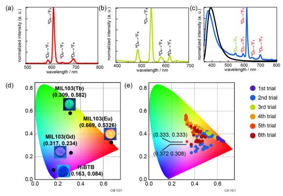
Fig. 2 Emission spectra at an excitation wavelength of 295 nm: (a) single MIL-103(Eu), (b) single MIL-103(Tb), and (c) single MIL-103(Gd) (blue) and organic ligand H<sub>3</sub>BTB (black). (d) CIE chromaticity diagram for single MIL-103(Eu, Gd, or Tb) and organic ligand H<sub>3</sub>BTB. (e) CIE chromaticity diagram for trial experiments 1-6.
