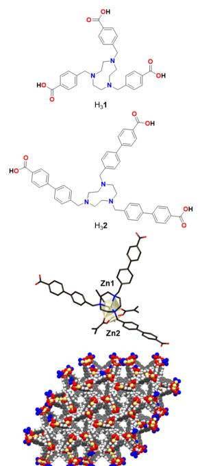
Fig. 1 Designed TACN-based tricarboxylic acid H<sub>3</sub>2 with extended, rigid arms compared to the previously reported H<sub>3</sub>1 (top), magnified view of the dinuclear Zn cluster in poly-[Zn<sub>2</sub>(2)(OH<sub>2</sub>)]Cl (middle), and view of the pore channels along the crystallographic c-axis (bottom).
