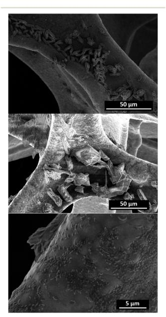
Fig. 4 SEM images of Co-TMBT-MOF/NF before (top) and after the 20 h (centre and bottom) OER tests in 1 M KOH at 20 mA cm $^{-2}$  and 23  $\pm$  2 °C.
