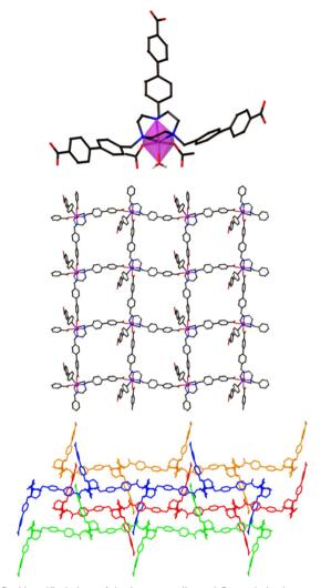
Fig. 2 Magnified view of the hexacoordinated Co node in the structure of poly- $[Co_2(H2)(OH_2)]\cdot 2DMF\cdot 4H_2O$  (top), simplified view of the framework viewed along the crystallographic a-axis (middle), and an expanded view to highlight how the sheets stack with interdigitation in the x direction (bottom).
