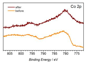
Fig. 5 High-resolution Co 2p XP spectra of the Co-TMBT-MOF/NF electrodes before and after the 20 h OER tests in 1 M KOH at 20 mA cm $^{-2}$  and 23  $\pm$  2 °C.
