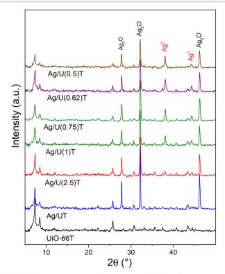
Fig. 3 XRD patterns of thermally-treated Ag/UiO-66 solids.
