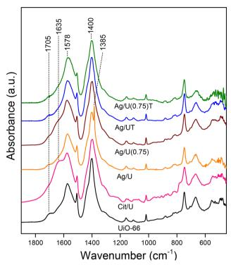
Fig. 1 FTIR spectra of Aq/UiO-66 solids prepared with different silver precursor/dispersant ratios (R). Spectra of some samples after heat treatment (T) are included.
