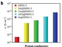
Fig. 11 (a) Schematic procedure of mechanochemically synthesized IM/MOF composite (b) the comparison of proton conductivity of the quest@NENU-3 composite and NENU-3 @338k. Reproduced with permission from ref. 1.
