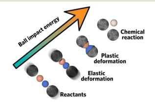
Fig. 1 Schematic procedures of mechanochemical ball milling. Reproduced with permission from ref. 3.
