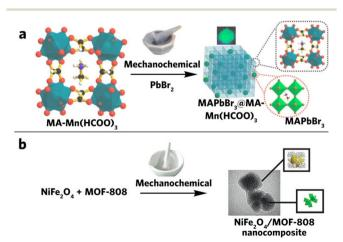
Fig. 8 (a) Synthesis of MAPbBr3@MA-Mn(HCOO)<sub>3</sub> via solvent-free mechanochemical grinding. Reproduced with permission from ref. 110, (b) mechanochemical synthesis of the NiFe<sub>2</sub>O<sub>4</sub>/MOF-808 composite. Reproduced with permission from ref. 111.
