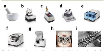
Fig. 3 Commonly used milling equipment. (a) Mortar and pestle, (b) automatic mortar, (c) vertical vibrational mini mill, (d) vibratory micromill. (e) vibrational ball mill. (f) vibrational ball mill with temperature control, (g) planetary ball mill, (h) multisampling mill, and (i) twin-screw continuous mechanochemical synthesis. Reproduced with permission from ref. 15.
