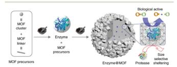
6 Two-step mechanochemical approach for embedding glycosidases into MOF. Reproduced with permission from ref. 24.
