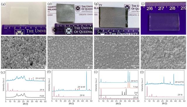
Fig. 9 Mechanochemical coating of ZIF-8 on various substrates: (a-c) one-pot coating on PVDF from ZIF-8 precursors, (d-f) one-pot coating on nickel foam (NF) from ZIF-8 precursors, (q-i) one-pot coating on Ti foils from ZIF-8 precursors, (j-l) ZIF-8 coating on FTO glass. Reproduced with permission from ref. 2.
