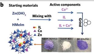
Fig. 10 (a) Mechanochemical deposition of gold clusters on porous coordination polymers. Reproduced with permission from ref. 100 (b) synthetic procedures of L@ZIF-8(Zn/Co). Reproduced with permission from ref. 133.
