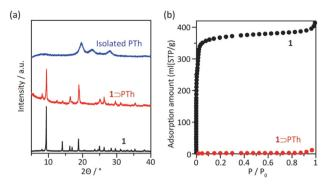
Fig. 3 (a) XRPD patterns of 1,  $1 \supset PTh$ , and PTh liberated from 1. (b)  $N_2$  adsorption isotherms of 1 and 1  $\supset$  PTh at 77 K (1;  $S_{BET}$  = 1447  $m^2 g^{-1}$ , 1  $\supset$  PTh;  $S_{BET} = 4 m^2 g^{-1}$ ).
