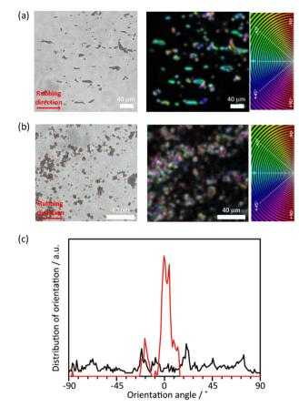
Fig. 6 (a and b) Microscope images and orientation analyses of (a) long and (b) short PTh rod particles after mechanical rubbing treatment. Orientation analyses were color-coded according to the orientation color map from -90° to +90°. (c) Angle orientation of the PTh rods with long (red) and short (black) length.
