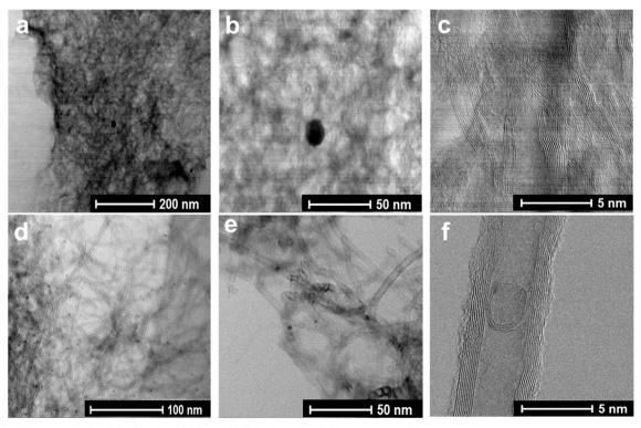
Fig. 3 BF-STEM images for (a-c) Fe<sub>1</sub>Co<sub>1</sub>-ZNT-900 and (d-f) Fe<sub>1</sub>Co<sub>2</sub>-ZNT-900 catalysts at different resolutions
