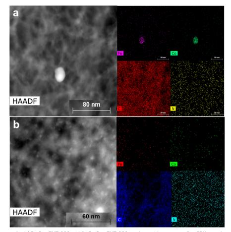
Fig. 4 HAADF-STEM images for (a) Fe<sub>1</sub>CO<sub>1</sub>-ZNT-900 and (b) Fe<sub>1</sub>CO<sub>2</sub>-ZNT-900 catalysts with corresponding EDX mapping.
