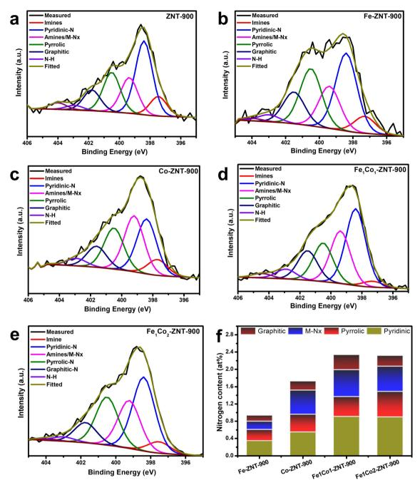
Fig. 5 (a-e) Comparison of N 1s XPS spectra for (a) ZNT-900, (b) Fe-ZNT-900, (c) Co-ZNT-900, (d) Fe<sub>1</sub>Co<sub>1</sub>-ZNT-900 and (e) Fe<sub>1</sub>Co<sub>2</sub>-ZNT-900 catalysts and (f) N content for different nitrogen groups.
