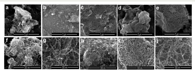
Fig. 2 SEM images captured for (a and f) ZNT-900, (b and g) Fe-ZNT-900, (c and h) Co-ZNT-900, (d and i)  $Fe_1Co_1$ -ZNT-900 and (e and j)  $Fe_1Co_2$ -ZNT-900 catalysts at different resolutions.
