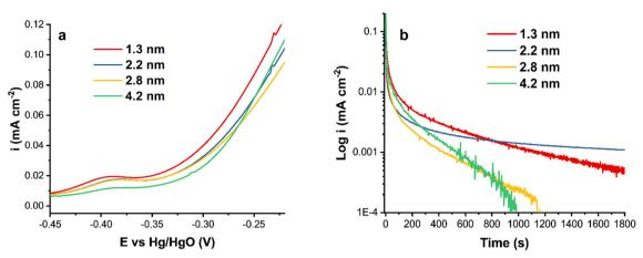
Fig. 3 (a) A comparison of the forward CV scans of Pt/C catalysts at v = 20 mV s<sup>-1</sup> and (b) chronoamperograms of Pt/C catalysts at -0.3 V in 1 M KOH + 0.5 M NH<sub>4</sub>OH.
