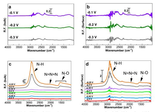
Fig. 6 PM-IRRAS spectra (considering KOH at -0.4 V as reference for processing the spectra) on Pt/C of 2.2 nm. (a and b) Spectra in 1 M KOH and (c and d) spectra in 1 M KOH + 0.5 M NH<sub>4</sub>OH. The applied potentials in (c) and (d), as indicated in the figure, are -0.5, -0.45, -0.45, -0.45, -0.45, -0.45, -0.45, and -0.25 V. The left hand side corresponds to the bulk of the electrolyte and the right hand side corresponds to the Pt surface.
