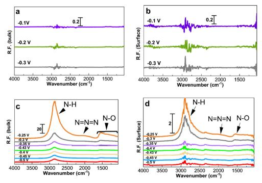
Fig. 5 PM-IRRAS spectra (considering KOH at -0.4 V as reference for processing the spectra) on Pt/C of 1.3 nm. (a and b) Spectra in 1 M KOH and (c and d) spectra in 1 M KOH + 0.5 M NH<sub>4</sub>OH. The applied potentials in (c) and (d), as indicated in the figure, are -0.5, -0.45, -0.45, -0.45, -0.45, -0.45, -0.45, and -0.25 V. The left hand side corresponds to the bulk of the electrolyte and the right hand side corresponds to the Pt surface.
