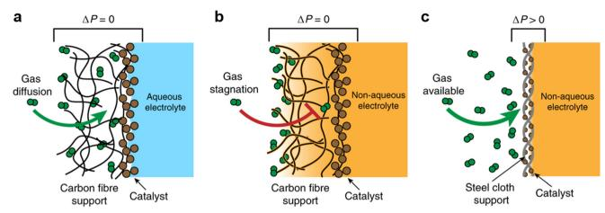
Fig. 10 (a) A hydrophobic GDE with an aqueous electrolyte; (b) a hydrophobic GDE with a non-aqueous electrolyte; (c) a catalyst-coated (SSC) GDE with a non-aqueous electrolyte.<sup>22</sup>
