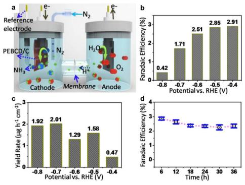
Fig. 11 (a) The graphic illustration of the configuration of the electrochemical cell for the eN<sub>2</sub>RR process; (b) FEs of the Li<sup>+</sup>-PEBCD/CC catalyst at different potentials during the eN<sub>2</sub>RR; (c) NH<sub>3</sub> yield rate against applied potential during the eN<sub>2</sub>RR; (d) durability test results for Li<sup>+</sup>-PEBCD/CC.<sup>3</sup>
