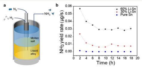
Fig. 9 (a) Graphical illustration of Li-eN<sub>2</sub>RR containing Li-Sn alloy and molten LiCl-KCl salt forming a biphasic system; (b) NH<sub>3</sub> yield rate against electrolysis time on Li-Sn and pure Sn.62
