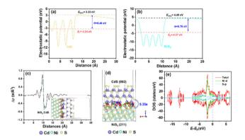
Fig. 4 Theoretical work functions of CdS (a) and NiS<sub>2</sub> (b). (c) Electron density difference (e  $Å^{-3}$ ) and (d) Bader electron transfer at the NiS<sub>2</sub>/CdS interfaces. (e) The density of states of NiS2.
