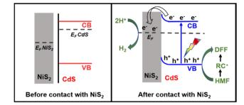
Scheme 2 Energy band diagrams of the pure CdS and NiS<sub>2</sub>/CdS before contact with metallic NiS2 and the interfacial photoinduced charge transfer and reaction after contact with NiS2 and light irradiation.
