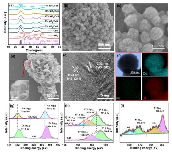
Fig. 2 (a) XRD patterns of the as-prepared CdS, x% NiS<sub>2</sub>/CdS, and NiS<sub>2</sub>; (b and c) SEM, (e) HRTEM, (f) element mapping images of the as-prepared 10% NiS<sub>2</sub>/CdS; (d) SEM of NiS<sub>2</sub>; (g-i) XPS spectra for CdS and 10% NiS<sub>2</sub>/CdS.
