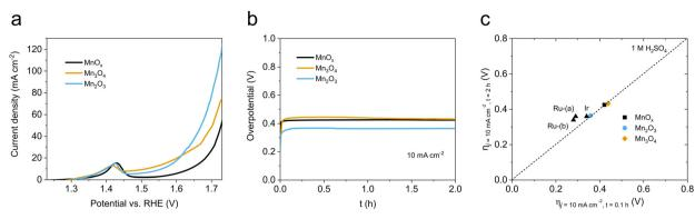
Fig. 3 (a) electrocatalytic activity of  $MnO_x/GPO$ ,  $Mn_3O_4/GPO$  and  $Mn_2O_3/GPO$ ; (b) stability tests of  $MnO_x/GPO$ ,  $Mn_3O_4/GPO$  and  $Mn_2O_3/GPO$  in chronopotentiometry measurements at 10 mA cm<sup>-2</sup>; (c) benchmarking of the activity/stability features between our Mn-based oxide and noble metal-based electrocatalysts according to the study of Jaramillo *et al.*<sup>6</sup>
