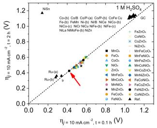
**Fig. 2** Benchmarking of the activity/stability features for OER electrocatalysts in acidic media following the protocol by Jaramillo *et al.*<sup>6</sup>
