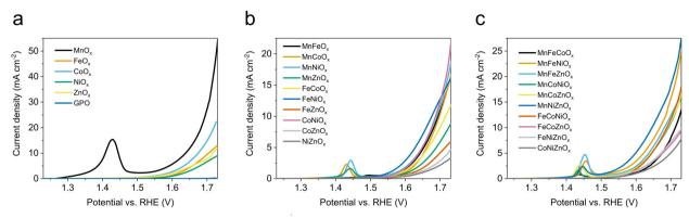
Fig. 1 LSV curves in 1 M H<sub>2</sub>SO<sub>4</sub> electrolyte (pH 0.1) with 1 mV s<sup>-1</sup> scan rate of (a) MO<sub>x</sub>/GPO, (b) MM'O<sub>x</sub>/GPO, (c) MM'M"O<sub>x</sub>/GPO.
