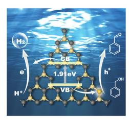
Fig. 7 Reaction mechanism of the photocatalytic hydrogen evolution coupled with benzyl alcohol oxidation for CCN-Pr $_{40}$ . Yellow: C, gray: N.
