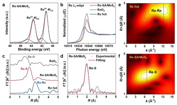
Fig. 3 (a) XPS spectrum of Re 4f in the Re-SA/MoS<sub>2</sub> catalyst. (b) XANES spectra of Re  $L_3$ -edge of Re foil, ReO<sub>2</sub> and Re-SA/MoS<sub>2</sub>. (c)  $k^3$ -weighted Re  $L_3$ edge Fourier-transformed EXAFS spectra for Re foil, ReO<sub>2</sub> and Re-SA/MoS<sub>2</sub>. (d) EXAFS spectra (experimental and fitting) of Re L<sub>3</sub>-edge of Re-SA/MoS<sub>2</sub>. (e) and f) Wavelet-transformation for Re L<sub>3</sub>-edge of Re foil and Re-SA/MoS<sub>2</sub> in R space
