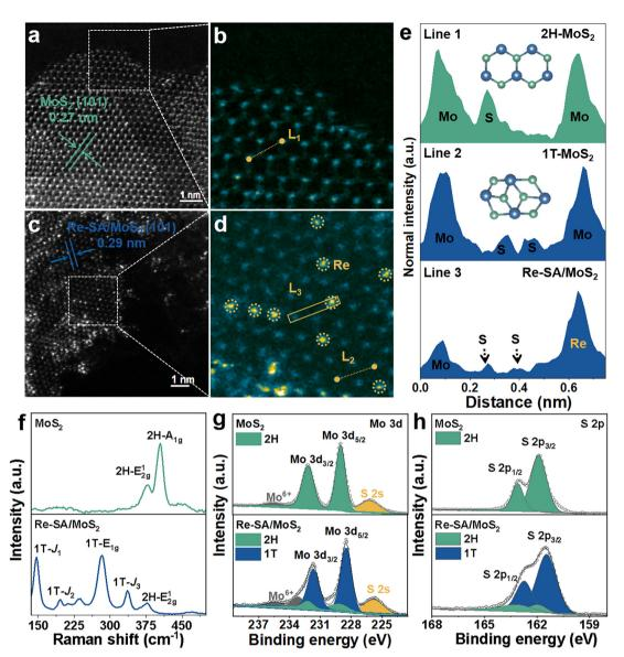
Fig. 2 (a and c) HAADF and (b and d) enlarged HAADF images of the 2H-MoS<sub>2</sub> and Re-SA/MoS<sub>2</sub> catalysts. (e) HAADF intensity line profiles taken along the numbered lines indicated in b and d. (f) Raman spectra of the fabricated  $MoS_2$  and  $Re-SA/MoS_2$  catalysts. (g and h) XPS spectra of the Mo 3d and S 2p of the fabricated MoS<sub>2</sub> and Re-SA/MoS<sub>2</sub> catalysts.
