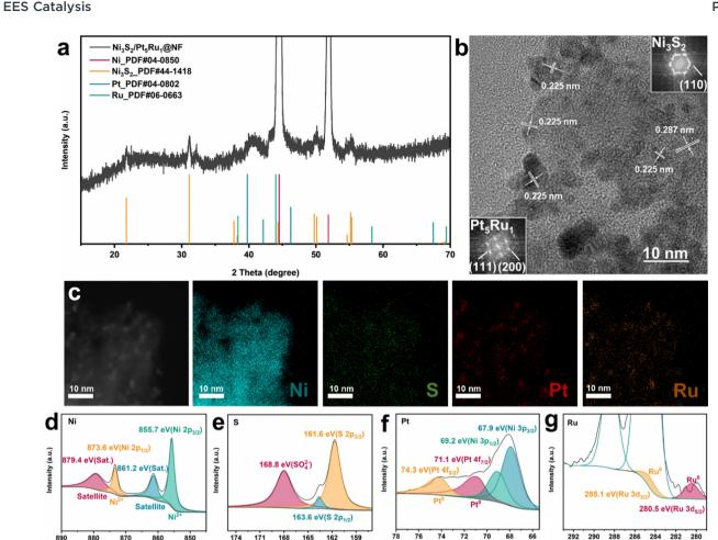
Fig. 1 Structural and microstructure characterizations of Ni<sub>3</sub>S<sub>2</sub>/Pt<sub>5</sub>Ru<sub>1</sub>@NF. (a) XRD pattern, (b) HRTEM image and the corresponding FFT patterns, (c) STEM image and the corresponding EDX elemental mapping images, and XPS spectra of (d) Ni 2p, (e) S 2p, (f) Pt 4f, and (g) Ru 3d.
