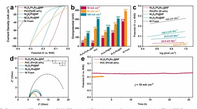
Fig. 3 Electrocatalytic HER performance in  $0.1 \,\mathrm{M}$  HClO<sub>4</sub> solution. (a) Polarization curves of the electrocatalysts for the HER (with 95% iR compensation), (b) the resultant overpotentials at current densities of 10, 50 and 100 mA cm<sup>-2</sup> for the as-prepared electrocatalysts, (c) the corresponding Tafel plots, (d) Nyquist plots under open-circuit voltage, and (e) long-term stability test at current densities of 10 mA cm<sup>-2</sup>.
