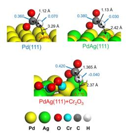
Fig. 7 Representative Mulliken atomic charges as determined by DFT calculations in reaction intermediate III for Pd(111), PdAq(111), and PdAg(111) associated with the Cr<sub>2</sub>O<sub>3</sub> cluster.
