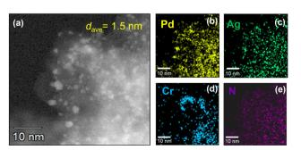
Fig. 1 (a) HAADF-STEM image of PdAgCr/amine-MSC. EDX mapping of (b) Pd, (c) Ag, (d) Cr, and (e) N over the region shown in (a).
