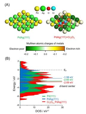
Fig. 4 (A) The optimized structure of pristine PdAg(111) and PdAg(111) associated with one stoichiometric Cr<sub>2</sub>O<sub>3</sub> cluster with a color overlay of representative Mulliken atomic charge determined using density functional theory calculations. (B) Calculated DOS plots.
