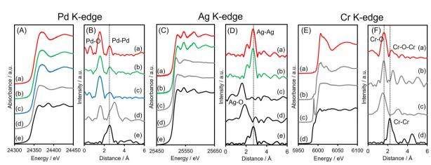
Fig. 3 (A) Pd K-edge XANES and (B) FT-EXAFS spectra of (a) PdAgCr/amine-MSC, (b) PdAg/amine-MSC, (c) Pd/amine-MSC, (d) PdO and (e) Pd foil; (C) Ag K-edge XANES and (D) FT-EXAFS spectra of (a) PdAgCr/amine-MSC, (b) PdAg/amine-MSC, (c) Ag<sub>2</sub>O, (d) AgNO<sub>3</sub> and (e) Ag foil; and (E) Cr K-edge XANES and (F) FT-EXAFS spectra of (a) PdAgCr/amine-MSC, (b) Cr<sub>2</sub>O<sub>3</sub>, (b) CrO<sub>3</sub>, and (c) Cr foil.
