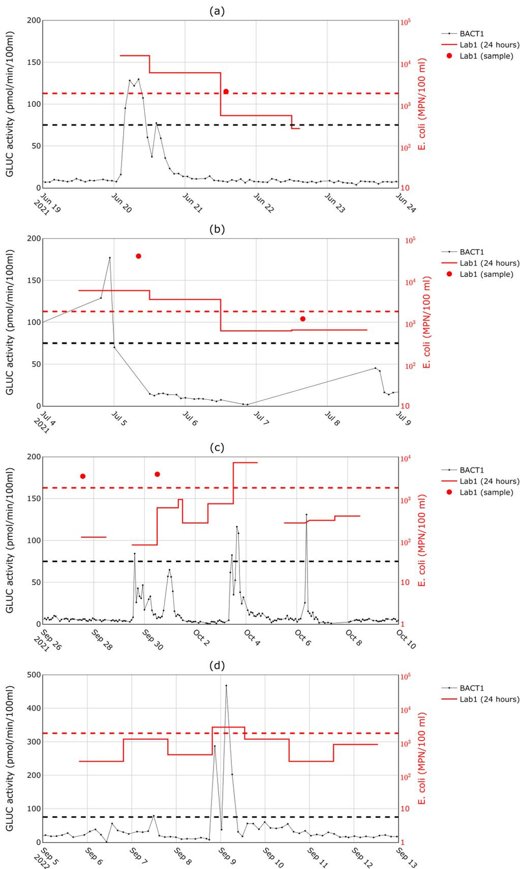
**Fig. 5** GLUC activity recorded by BACTcontrol (left axis) and *E. coli* concentration measured via the MPN method (right axis) during four different overflow events: a) 19–24 June 2021, b) 4–9 July 2021, c) 26 September – 10 October 2021, and d) 5–13 September 2022. The red and black dashed lines show the established hygienic limit values for *E. coli* and GLUC activity, respectively.
