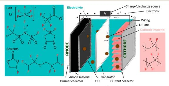
Fig. 1 Simplified schematic of a lithium-ion battery, adapted from Bresser et al. (2015),<sup>38</sup> including examples of fluorinated species included in many batteries, some of which are classified as PFAS under the OECD definition.
