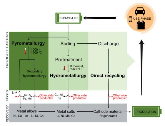
Fig. 3 Overview of handling, material losses, and material recovery for the three major LIB recycling processes: pyrometallurgy, hydrometallurgy and direct recycling. Temperatures are  $\cong$  ambient when not stated. Dashed arrows indicate fractions that are not possible to recycle using a given process. Figure adapted from Kushnir, 2015 <sup>86</sup> and Lv *et al.*, 2018.<sup>83</sup>
