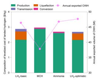
Fig. 11 Comparison of average LCOH<sup>L</sup> and annual exported volume of OWH via liquid hydrogen, methylcyclohexane (MCH), and ammonia shipping in 2050
