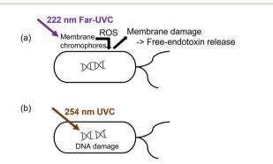
Fig. 2 Possible different inactivation mechanisms between (a) 222 nm and (b) 254 nm that affect the increase in EAR.
