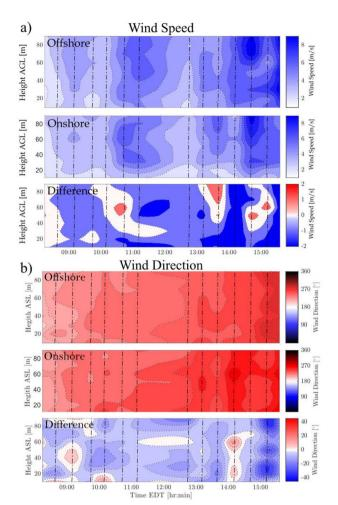
Fig. 10 2-D contour plots showing the comparison of onshore and offshore profiles of (a) wind speed and (b) wind direction measured on August 6th. The dashed lines show the sUAS flights.
