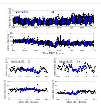
Fig. 5 Comparison plots showing the agreement between the multirotor sUAS (blue dots) and sonic anemometer (SA; black dots) measurements of wind speed and wind direction collected on August 8th from (a) 8:00 to 15:00 EDT, as well as periods of (b) light (U < 3 m s<sup>-1</sup>) and (c) moderate (U < 5 m s<sup>-1</sup>) wind conditions.
