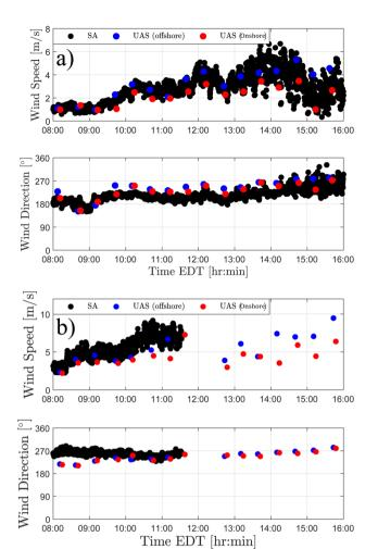
Fig. 8 Comparison plots showing differences between multirotor sUAS estimates of wind speed and wind direction at onshore (red) and offshore (blue) locations 10 m AGL on the (a) 5th and (b) 6th of August. The black markers correspond to the sonic anemometer (SA) observations collected 13 m AGL on August 5th and 6th.
