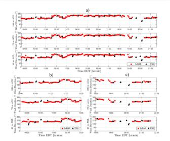
Fig. 7 (a) A comparison plot showing the agreement between multirotor sUAS (black) and SoDAR (red) wind direction observations collected at 40 m, 70 m, and 100 m AGL on June, 27th, 2020. Multirotor and SoDAR wind direction observations were found in good agreement consistently during the (b) morning and (c) evening sampling periods.
