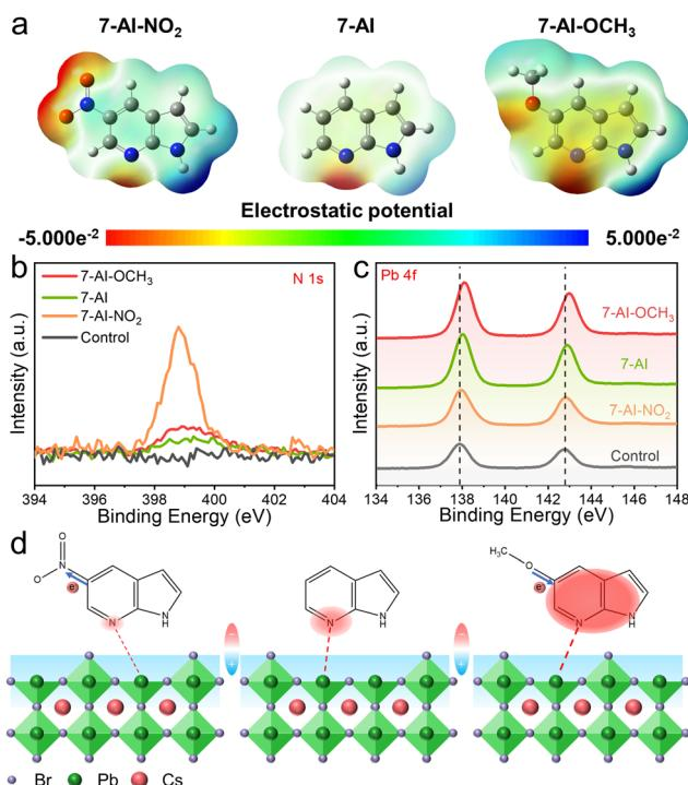
**Fig. 1** (a) Molecular structures and electrostatic potential maps of 5-nitro-7-azaindole (7-AI- $NO_2$ ), 7-azaindole (7-AI), and 5-methoxy-7-azaindole (7-AI- $OCH_3$ ). XPS spectra of (b) N 1s and (c) Pb 4f in  $CsPbBr_3$  films without and with organic molecule treatment. (d) Schematic diagram of electron-transfer-induced coulomb force regulation and the N atom passivated uncoordinated  $Pb^{2+}$ .
