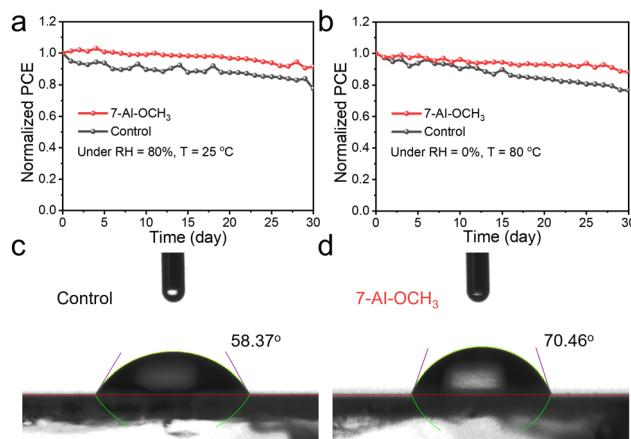
**Fig. 4** Long-term stability of the inorganic CsPbBr<sub>3</sub> PSCs at (a) RH = 80%, T = 25 °C and (b) RH = 0%, T = 80 °C. The water contact angle of (c) control and (d) 7-Al-OCH<sub>3</sub>-based perovskite films.
