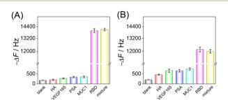
Fig. 4 Selectivity of the HF-QCM aptasensor (A) and immunosensor (B) for the RBD assay. RBD, 100 pg mL<sup>-1</sup>; interferent, 1 ng mL<sup>-1</sup>; the mixture contained the RBD (100 pg mL<sup>-1</sup>) and four interferents (each interferent,  $1 \text{ ng mL}^{-1}$ ).
