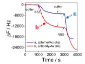
Fig. 2 Real-time responses of the aptamer (antibody)-modified QCM Au chip for the following processes: washing with buffer, blocking the surface with BSA, washing with buffer, and specific recognition of the RBD.  $C_{RBD} = 100 \text{ pg mL}^{-1}$ .
