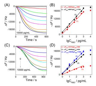
Fig. 3 Frequency changes of the HF-QCM aptasensor (A) and immunosensor (C) with different concentrations of the RBD: 0, 1, 5, 10, 50, 100, 500, 1000, and 10 000 pg mL<sup>-1</sup>. Dependence of  $-\Delta F$  values of the HF-QCM aptasensor (B) and immunosensor (D) at definite recognition times on the logarithm of RBD concentrations.
