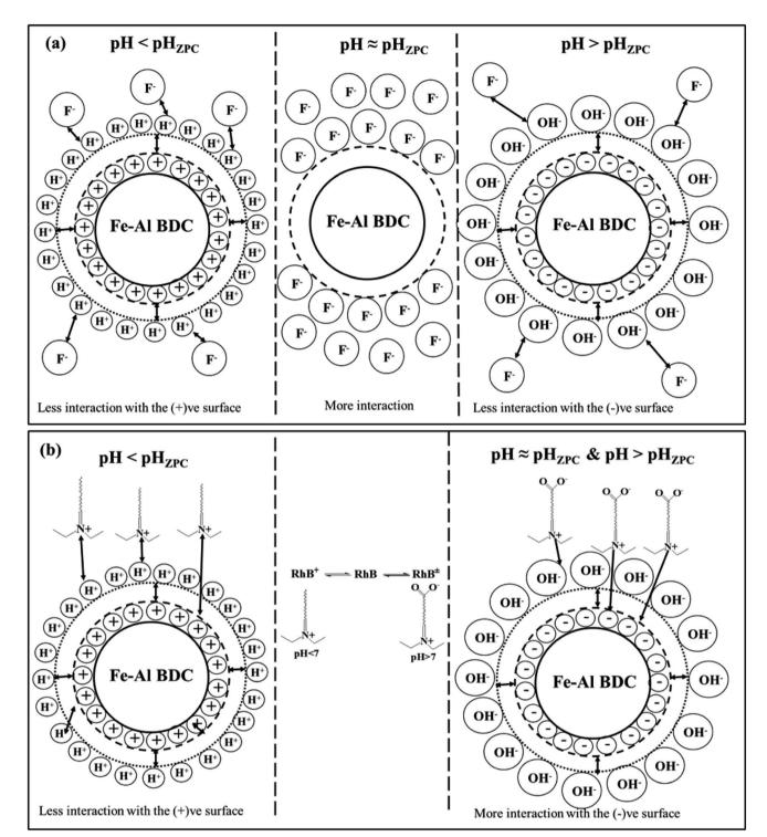
Fig. 8 A schematic representation of the surface-boundary-layer mechanism using the electrical double layer model for (a) F<sup>-</sup> adsorption and (b) the photodegradation of RhB in different pH media onto an Fe-Al BDC surface prepared at 473 K for 70 h.
