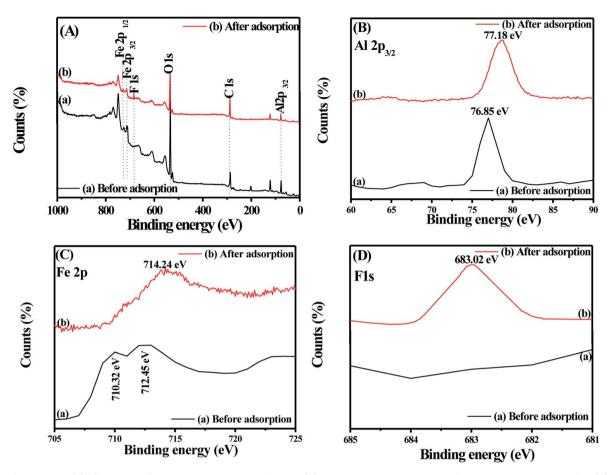
Fig. 9 XPS spectra of (A) (a) Fe-Al BDC prepared at 473 K for 70 h and (b) fluoride-adsorbed Fe-Al BDC prepared at 473 K for 70 h; (B) Al  $2p_{3/2}$  area analysis (a) before fluoride adsorption and (b) after fluoride adsorption; (C) Fe  $2p_{3/2}$  area analysis (a) before fluoride adsorption and (b) after fluoride adsorption and (b) after fluoride adsorption at pH 7.
