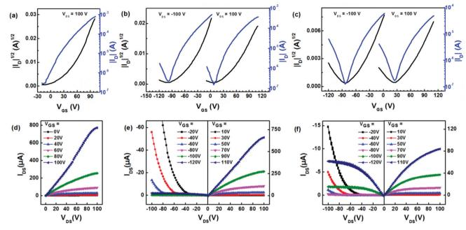
Fig. 4 The transfer (a-c) and output (d and f) characteristics of the field-effect transistors based on three polymers measured under optimized conditions. (a and d) PNBDO-TT. (b and e) PNBDO-DMTT. (c and f) PNBDO-MOTT.
