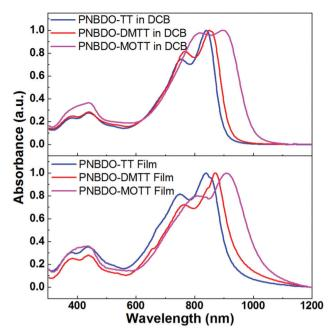
Fig. 1 UV-vis-NIR absorption spectra of the three thienothiophenebisoxoindolinylidene-benzodifurandione copolymers in DCB solutions and thin films
