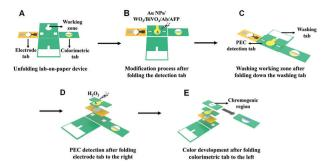
Fig. 1 (A–E) Assembly and operation illustration of the lab-on-paper device. (A) Unfolding the lab-on-paper device. (B) Modification process after folding the detection tab. (C) Washing working zone after folding down the washing tab. (D) PEC detection after folding the electrode tab to the right. (E) Color development after folding the colorimetric tab to the left
