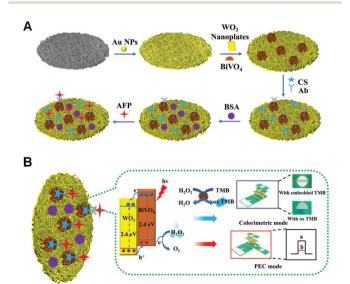
Scheme 1 (A) Fabrication procedure of the lab-on-paper PEC sensing platform. (B) Schematic illustration of the PEC/colorimetric analytical principle. (Colorimetric mode: the folding state of the lab-on-paper device shown in blue rectangle and the colorimetric results before and after incubation of AFP; PEC mode: the folding state of the lab-on-paper device shown in red rectangle and the PEC signal before and after incubation of
