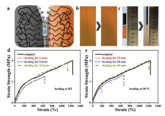
Fig. 4 Self-healing properties of the ionogel: (a) illustration of the selfhealing mechanism; (b) POM photos of the ionogel before and after selfhealing; (c) qualitative tensile photos of ionogel before and after self-healing; (d and e) the tensile curves of the ionogel healing at room temperature or 50 °C for different time
