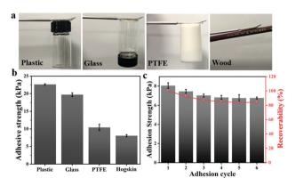
Fig. 5 The adhesion properties of the ionogel: (a) photos of the ionogel on the surface of various substrates including plastic, glass, PTFE, and wood; (b) quantification of the adhesion of ionogels to different object surfaces; (c) repeatable adhesion behavior of the ionogel to hogskin.
