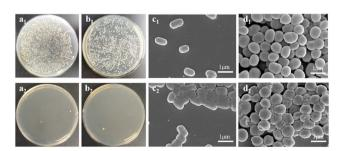
Fig. 7 Characterizations of antibacterial ability: (a and b) two kinds adhered viable bacterial of pure PU and ionogel against E. coli and S. aureus; (c and d) SEM photos of E. coli and S. aureus after incubating with pure PU and ionogel.
