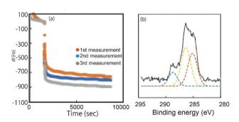
Fig. 2 Glycopolymer layer formation by adsorption of thiol-terminated pMan<sub>200</sub>. (a) Time course of frequency change of three different measurements in QCM by the adsorption of  ${\bf pMan_{200}}$  with 10 g  ${\rm L^{-1}}$  at 15 C for 2 h. (b) XPS C (1s) spectrum of pMan<sub>200</sub> immobilized substrate after the adsorption of the glycopolymer and water rinsing.
