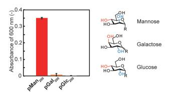
Fig. 4 Turbidity measurement of pMan<sub>200</sub>, pGal<sub>200</sub> and pGlc<sub>200</sub> and the chemical structure of monosaccharides. Turbidity of each glycopolymer was measured after dissolution in HEPES buffer at 1 g L<sup>-1</sup> and standing at 15 °C for 48 h.
