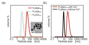
Fig. 5 (a) DLS measurement of  $P_{90}Man_{200},\,P_{90}Gal_{200}$  and  $P_{90}Glc_{200}$  and the TEM image of  $P_{90}Man_{200}$  (inset). (b) DLS measurement of  $P_{90}Man_{200}$ with (red) and without (black) Ca2+
