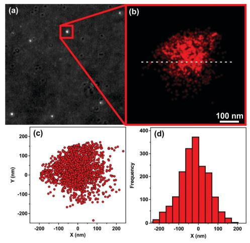
Fig. 2 Transmitted light image of the particles on a glass surface (a) and dSTORM picture of the marked focal point (b). Blinking events of the fluorophores were plotted along the X and Y axes (c) and the frequency of blinking events was plotted as a function of the distance (d) from the white dashed line shown in (b)
