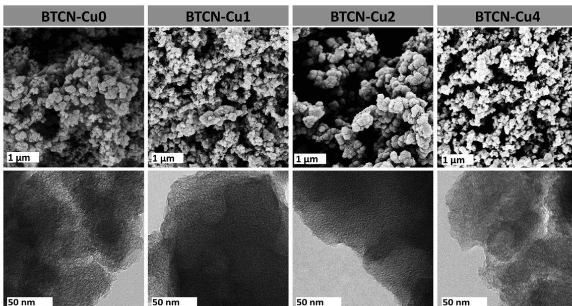
**Fig. 2** Micrographs of BTCN-Cu<sub>0</sub>, BTCN-Cu<sub>1</sub>, BTCN-Cu<sub>2</sub> and BTCN-Cu<sub>4</sub>. Top row: surface morphology visualized by SEM, using a secondary electron detector. Bottom row: overview TEM images.
