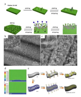
Fig. 16 (a) Electro-plating/stripping process of pristine zinc and the 3D dual-channel porous Zn. Adapted from ref. 154. Copyright 2020, Elsevier. SEM images of (b) CNT and (c) Zn/CNT. (d) Electric field distribution models for the Zn-CC and Zn-CNT anodes after zinc nucleation. (e) Illustration of zinc plating on Zn-CC and Zn-CNT anodes. Adapted from ref. 155. Copyright 2019, Wiley-VCH.
