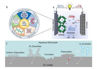
Fig. 1 (a) Schematic illustration of the working principle of ZIBs. Adapted from ref. 11. Copyright 2020, *Chem. Soc. Rev.* (b) Representative cathode materials. Adapted from ref. 16. Copyright 2021, Wiley-VCH. (c) Schematic diagram of interactions with aqueous electrolyte on the zinc anode surface.
