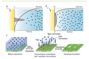
Fig. 4 Schematic plots are shown for gradients in the ion concentration in (a) a strong concentration gradient and (b) a mild concentration gradient with corresponding metal morphologies near the electrode surface. Adapted from ref. 53. Copyright 2019, AAAS. (c) Illustration of the effect of concentration polarization on zinc deposition. Adapted from ref. 40. Copyright 2022, Wiley-VCH.
