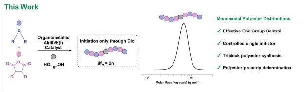
Fig. 1 ROCOP catalysts usually have a mixture of initiators resulting in bimodal polyester molar mass distributions.<sup>30</sup> This work describes an organometallic complex, applied with diol, which yields high molar mass, monomodal polyester distributions.
