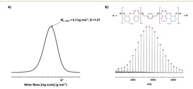
Fig. 2 (A) Molar mass distribution of poly(vinyl cyclohexene phthalate) (PvCHPE) obtained with complex 1. Conditions: [1]: [BDM]: [PA]: [vCHO] = 1:4:100:2000,  $T=100\,^{\circ}\text{C}$ . (B) MALDI-ToF spectrum of PvCHPE obtained.  $M_{n,calc}$  (repeat unit) = 272.3 g mol $^{-1}$ ,  $M_{n,theoretical}$  (repeat unit) = 272.3 g mol $^{-1}$ ;  $M_{n,calc}$  (end group = BDM + K $^{+}$ ) = 177.4 g mol $^{-1}$ ,  $M_{n,theoretical}$  (end group) = 177.3 g mol $^{-1}$ .
