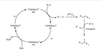
Scheme 3 Proposed reaction mechanism for the visible light-mediated ATRA reaction via reductive quenching of the excited state of  $[Fe(btz)_3](PF_6)_3$  1.
