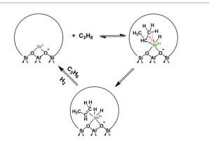
Scheme 1 Schematic of proposed mechanisms for PDH on isolated In+ sites.
