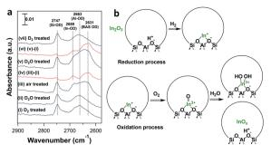
Fig. 8 (a) FTIR spectra of reduced In-CHA(11, 1.0) treated under different conditions at 550 °C: (i)  $D_2$ ; (ii)  $D_2O$ ; (iii) air; (iv) (i) subtracted from the spectrum (iii); (v)  $D_2O$ ; (vi) (i) subtracted from the spectrum (v); (vii)  $D_2O$ . Background spectrum was collected in the spectral cell with the  $H_2$  reduced sample pellet at 550 °C. (b) Proposed structures of exchanged In species in In-CHA upon reduction and subsequent oxidation.
