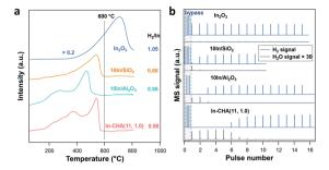
Fig. 2 (a)  $\rm H_2$ -TPR profiles and (b) results of  $\rm H_2$  pulse experiments on In-based catalyst at 600 °C.
