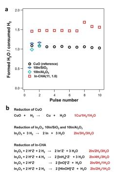
Fig. 3 (a) Determination of the formed  $H_2O$ /consumed  $H_2$  ratio from  $H_2$  pulses as a function of pulse number on several catalysts. (b) Stoichiometric analysis during reduction on CuO,  $In_2O_3$ ,  $10In/SiO_2$ , and  $10In/Al_2O_3$ , and potential reactions on In-CHA catalysts.
