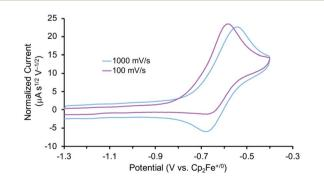
Fig. 3 Cyclic voltammogram of the first oxidation of 3 (0.2 mM) in 0.2 M NBu<sub>4</sub>PF<sub>6</sub> solution in THF under N<sub>2</sub> using a glassy carbon working electrode, Pt wire auxiliary electrode, and Ag wire pseudoreference. Potentials referenced to Cp<sub>2</sub>Fe<sup>+/0</sup> after the experiments.
