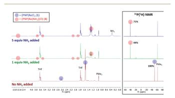
Fig. 2  $^{1}$ H and  $^{31}$ P{ $^{1}$ H} NMR spectra of 1 in THF- $d_{8}$  without NH $_{3}$  (bottom, maroon), with 1 equiv. NH $_{3}$  added (middle, green), and with 5 equiv. NH $_{3}$  added (top, blue). Spectroscopic yields reported vs. PMe $_{3}$  in a capillary.
