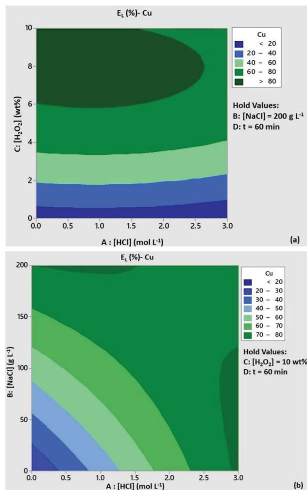
Fig. 2 Contour plots of Cu leaching efficiency as a function of (a) [HCl]/[H<sub>2</sub>O<sub>2</sub>] and (b) [HCl]/[NaCl]. Conditions: L/S = 10 mL g<sup>-1</sup>, *T* = 80 °C, *t* = 60 min and (a) [NaCl] = 200 g L<sup>-1</sup>, (b) [H<sub>2</sub>O<sub>2</sub>] = 10 wt%.
