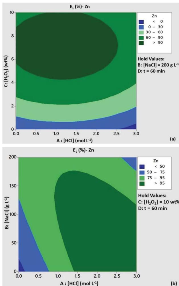
Fig. 3 Contour plots of Zn leaching efficiency as a function of (a)  $[HCl]/[H_2O_2]$  and (b)  $[HCl]/[NaCl]$ . Conditions:  $L/S = 10$  mL g<sup>-1</sup>,  $T = 80$  °C,  $t = 60$  min and (a)  $[NaCl] = 200$  g L<sup>-1</sup>, (b)  $[H_2O_2] = 10$  wt%.
