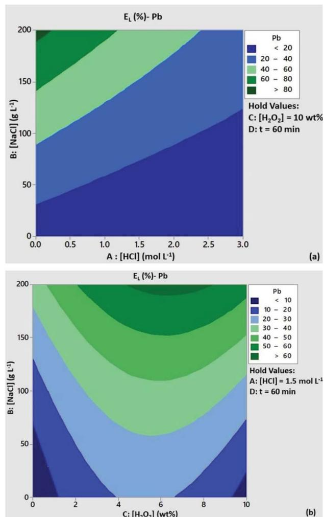
Fig. 4 Contour plots of Pb leaching efficiency as a function of (a)  $[HCl]/[NaCl]$  and (b)  $[H_2O_2]/[NaCl]$ . Conditions:  $L/S = 10$  mL g<sup>-1</sup>,  $T = 80$  °C,  $t = 60$  min and (a)  $[H_2O_2] = 10$  wt%, (b)  $[HCl] = 1.5$  mol L<sup>-1</sup>.
