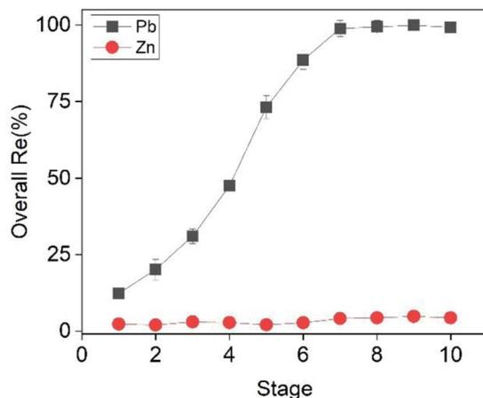
Fig. 8 Effect of ion flotation stage on the recovery efficiency of Pb and Zn. Conditions:  $[\text{Zn}]_i = 22.5 \text{ mmol L}^{-1}$ ,  $[\text{Pb}]_i = 3.5 \text{ mmol L}^{-1}$ ,  $[\text{CTAB}]_{\text{total}} = 9 \text{ mmol L}^{-1}$  ( $0.9 \text{ mmol L}^{-1}$  per stage),  $t_{\text{total}} = 50 \text{ min}$  (5 min per stage)  $[\text{EtOH}] = 0.5\% \text{ (v/v)}$ ,  $V = 50 \text{ mL}$ , flowrate =  $25 \text{ mL min}^{-1}$ .
