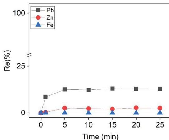
Fig. 7 Effect of ion flotation time on the recovery efficiency of Zn, Pb and Fe from the PLS after the cementation step. Conditions: [CTAB] =  $0.9 \text{ mmol L}^{-1}$ ,  $[\text{Zn}]_i = 22.5 \text{ mmol L}^{-1}$ ,  $[\text{Pb}]_i = 3.5 \text{ mmol L}^{-1}$ ,  $[\text{Fe}]_i = 500 \text{ mmol L}^{-1}$ , [EtOH] = 0.5% (v/v),  $V = 50 \text{ mL}$ , flowrate =  $25 \text{ mL min}^{-1}$ .
