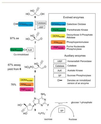
Fig. 3 Biocatalytic synthesis of islatravir. (This figure has been adapted from ref. 22. With permission from Science Journal, copyright 2020).
