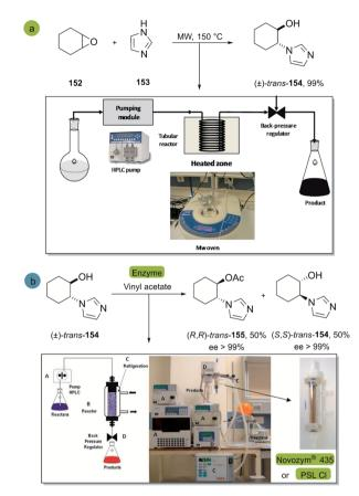
Scheme 22 Synthesis of trans-2-(1H-imidazol-1-yl)cyclohexanol (b) enantioselective acylation of ( $\pm$ )-trans-2-(1H-imidazol-1-yl)cyclohexanol 154 with vinyl acetate catalyzed by Novozym® 435 or PSL-CI. This figure was used with permission.
